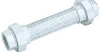
Application : Absorption of the piping strain in the line of water, steam,oil, chemicals, etc., absorption of vibration and groud sinking. Max. Working Temperature : 220°C
